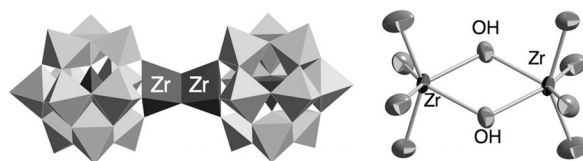
Figure 18. Polyhedral representation [\{\text{PW}_{11}\text{O}_{39}\text{Zr}(\mu\text{-OH})_2\}_2]^{8-} and the structure of the dinuclear \text{Zr}^{\text{IV}} cluster moiety. [30]
